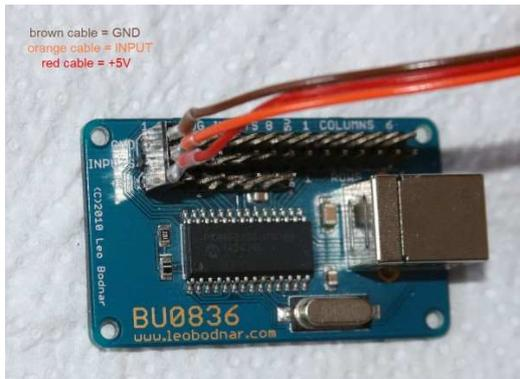
So, if all sensors are connected, all red wires must be on the same side corresponding with the [+5V] label.
